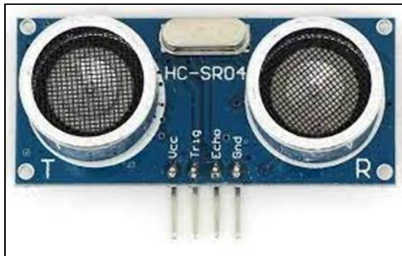
Figure 1: The HC-SR04 Sensor Is Used for Distance Sensing Using Ultrasonic Sound Waves
