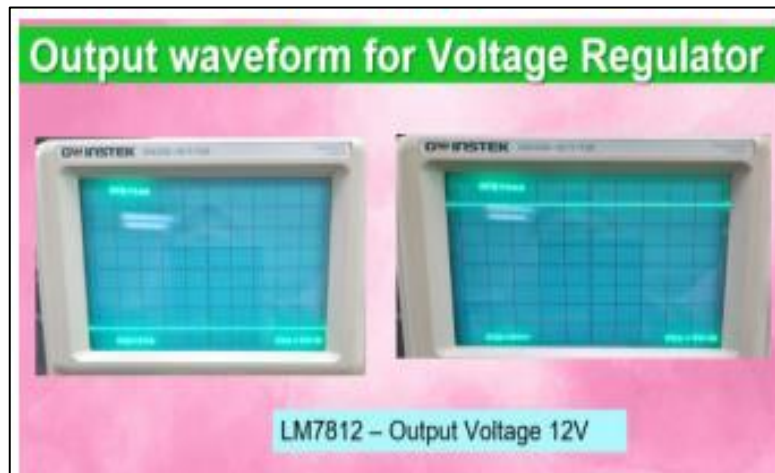
Figure 3.4 Output waveform for regulator
