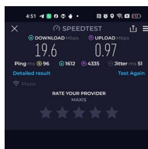
Figure 8: Speed Test reading after installing the Yagi Antenna
