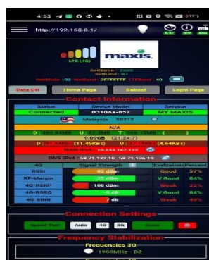
Figure 10: Analyze Huawei Manager after installing the Yagi Antenna
