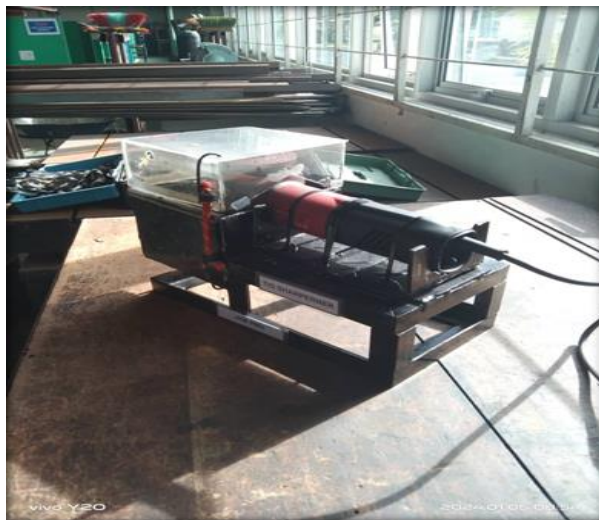
Figure 3:3 Tungsten Sharpener using hand grinder jig
