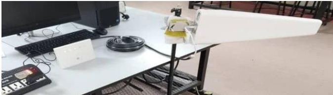
Figure 2: Antenna Connection on Huawei Modem Router to an external antenna (Yagi Antenna).
