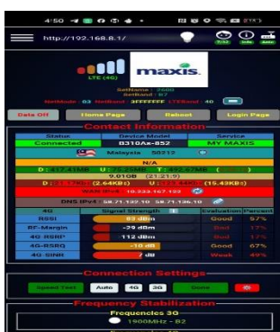
Figure 9: Analyze Huawei Manager before installing the Yagi Antenna
