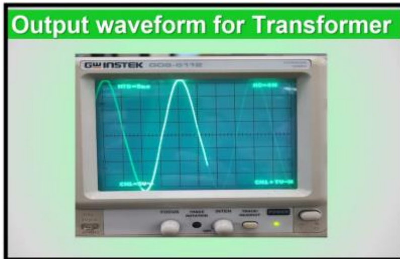
Figure 3.1 Output waveform for center-tap transformer
